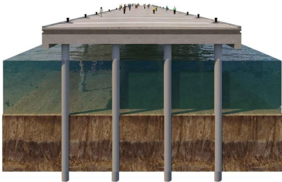
Image Caption: CBF Cross Sectional View Showing Pilings
