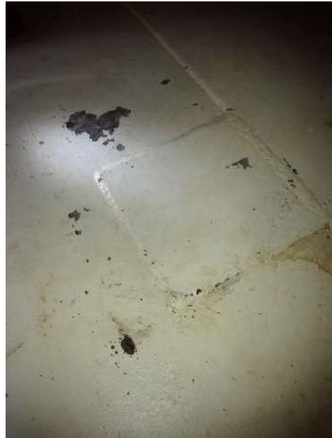
Tank #32198 Bottom Plate Failure
