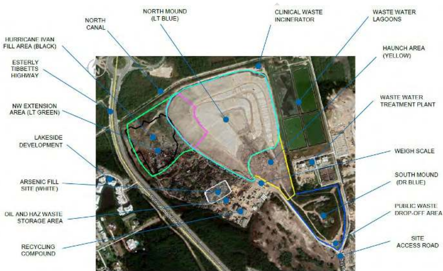
Figure 9.4 Layout of the George Town Landfill according to GHD (2020) 69
