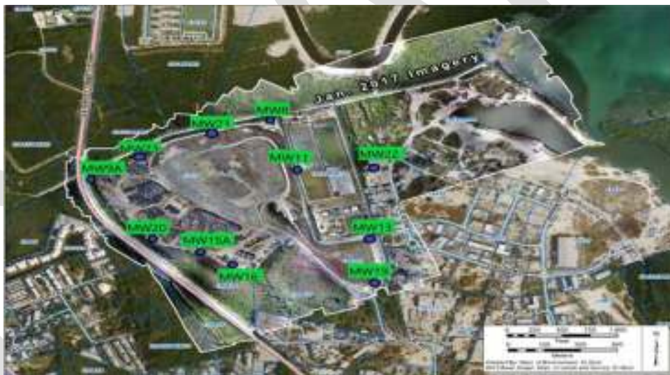
Figure 9.11 Location of groundwater monitoring wells at the GTLF (After Figure 1 in EHL 93 )
