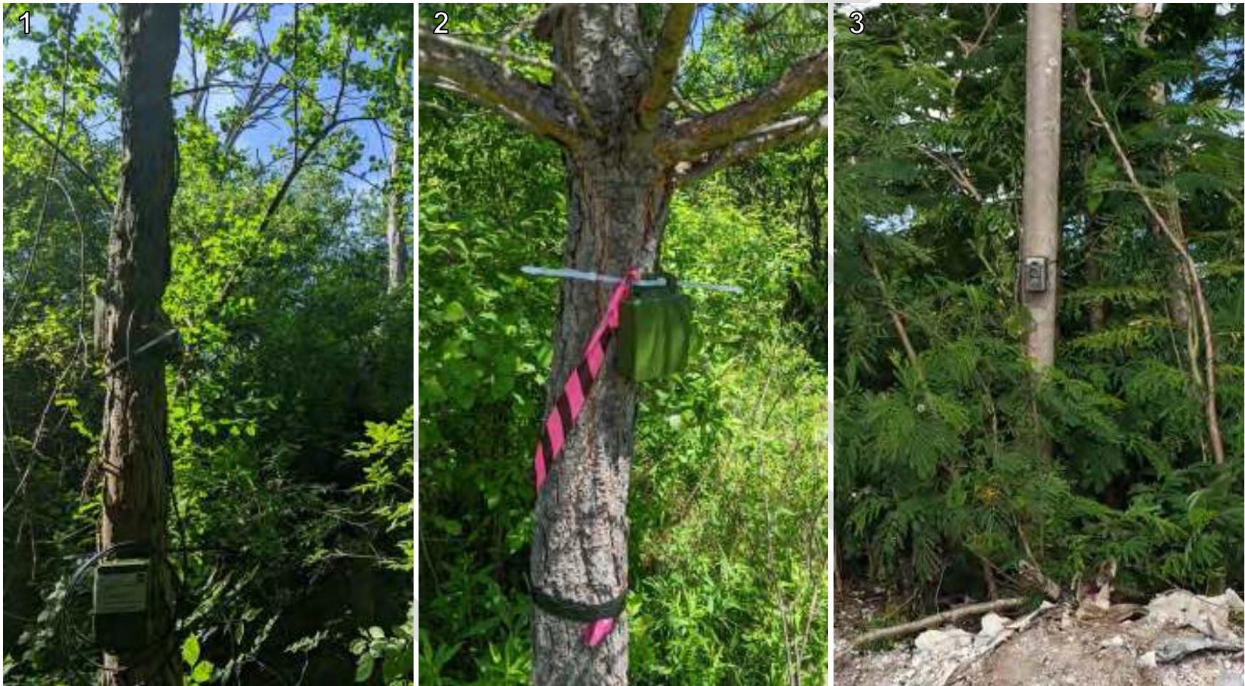
Figure 7.3 Terrestrial Ecology wildlife survey equipment set-ups: (1) bat acoustic survey, (2) audiofauna survey, and (3) wildlife camera survey
