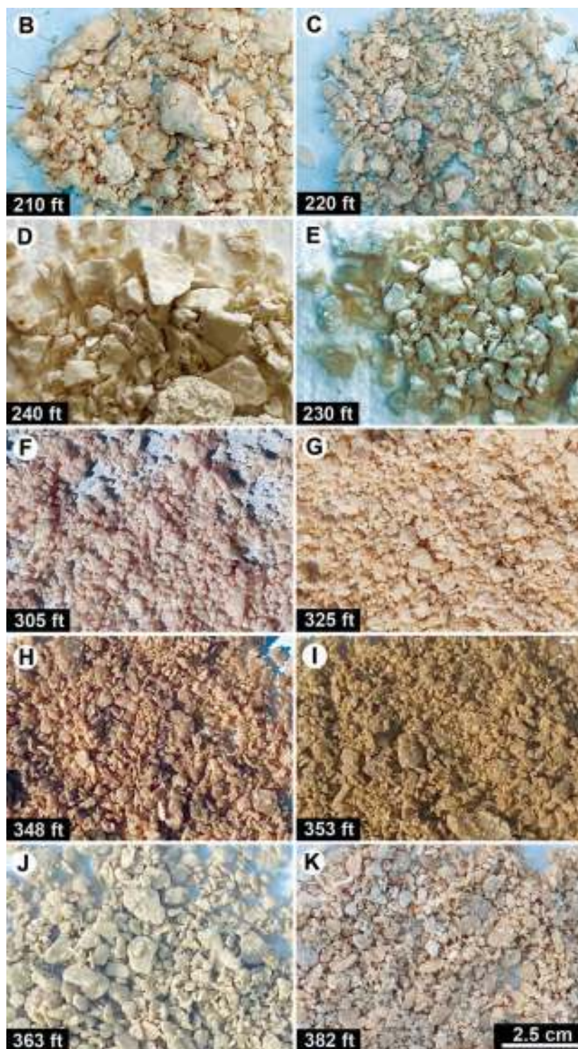
Figure 16: (A) Drill times for DUM-1 from 200 ft to base of well and locations of cores 1 to 4), insets show a segment of each core for comparative purposes. (B-K) Photographs of cuttings at various depths between 210 ft and 382 ft. Boundary between the Cayman Formation and Brac Formation lies somewhere between core 1 and core 2.
