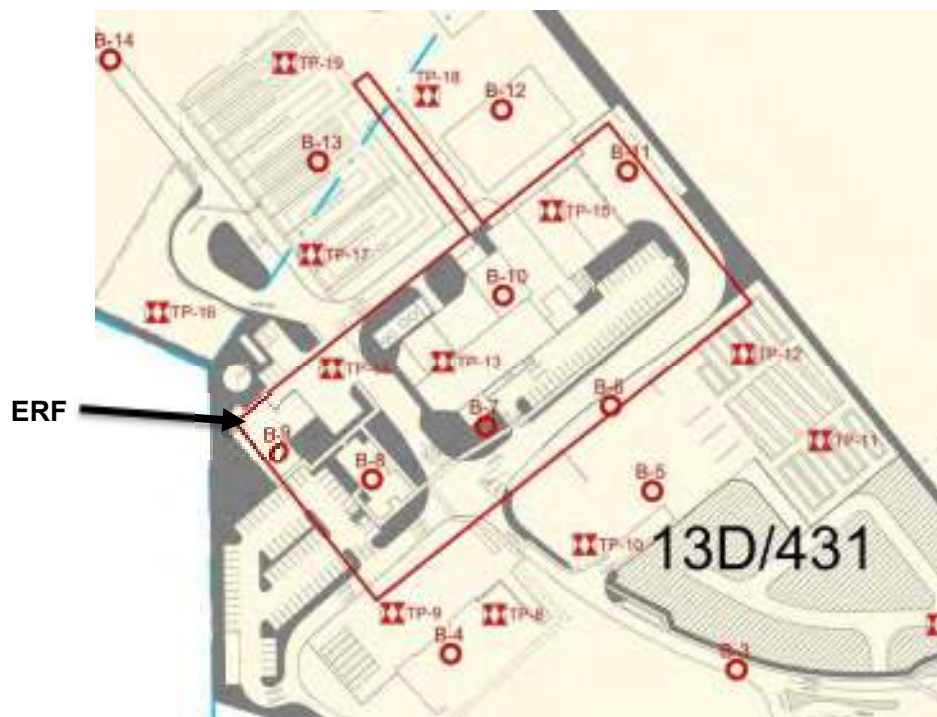
Figure 11 – Approximate Locations of Trial Pits & Boreholes
