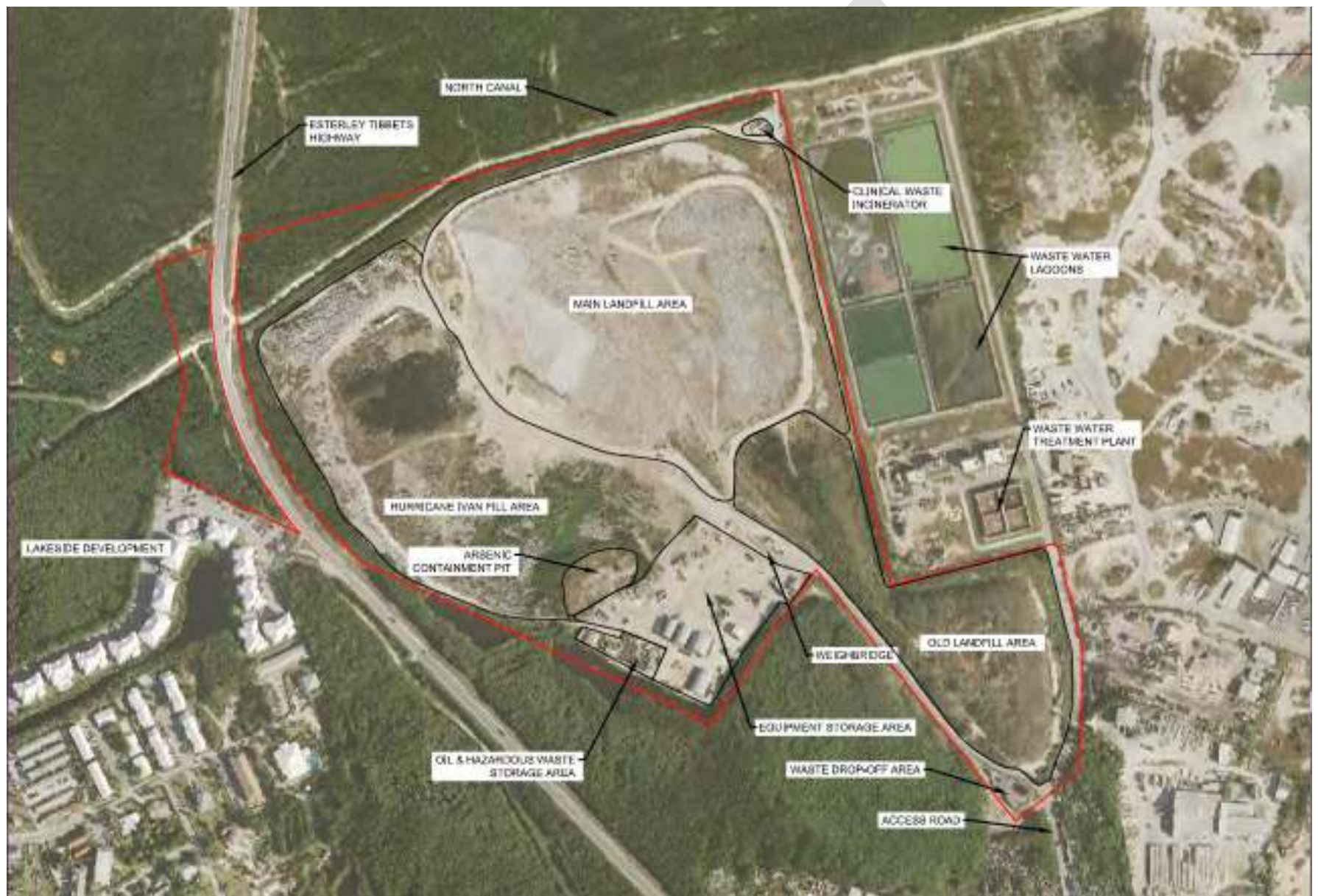
Figure 9.3 Boundary and layout of the George Town Landfill according to Amec Foster Wheeler 68
