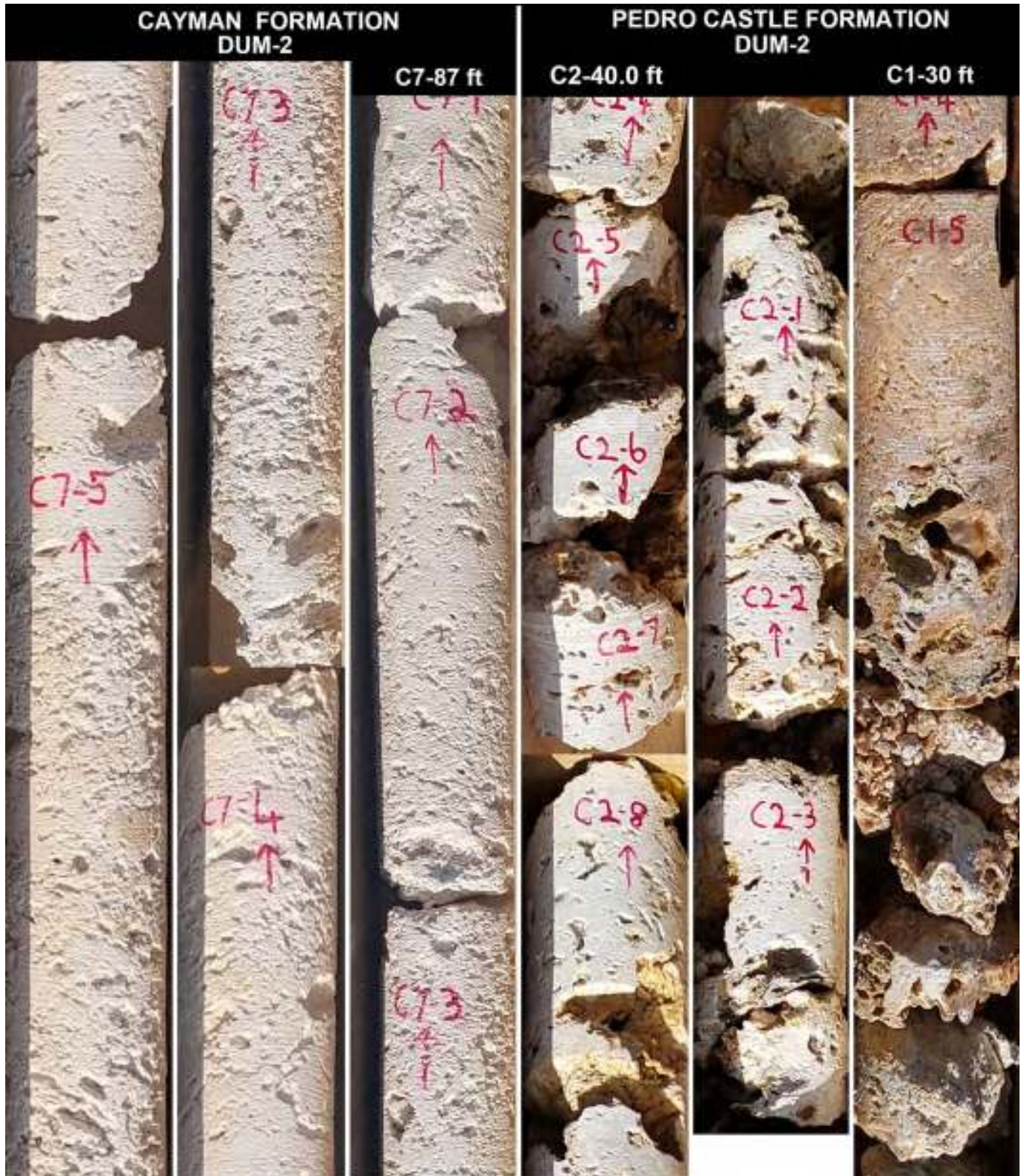
Figure 13: Comparison of cores from the Pedro Castle Formation C1 and C2) and cores from the Cayman Formation (C5-7) from DUM-2. Note higher porosity and shorter core pieces from the Pedro Castle Formation relative to the Cayman Formation. Core diameter is 4 in (10 cm).
