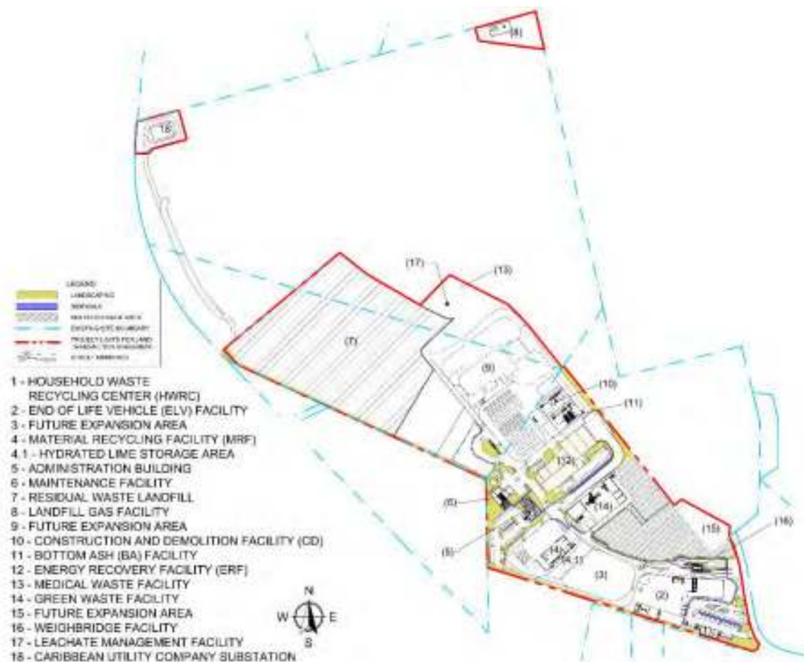
Figure 17 - Proposed Integrated Solid Waste Management Facility Layout
