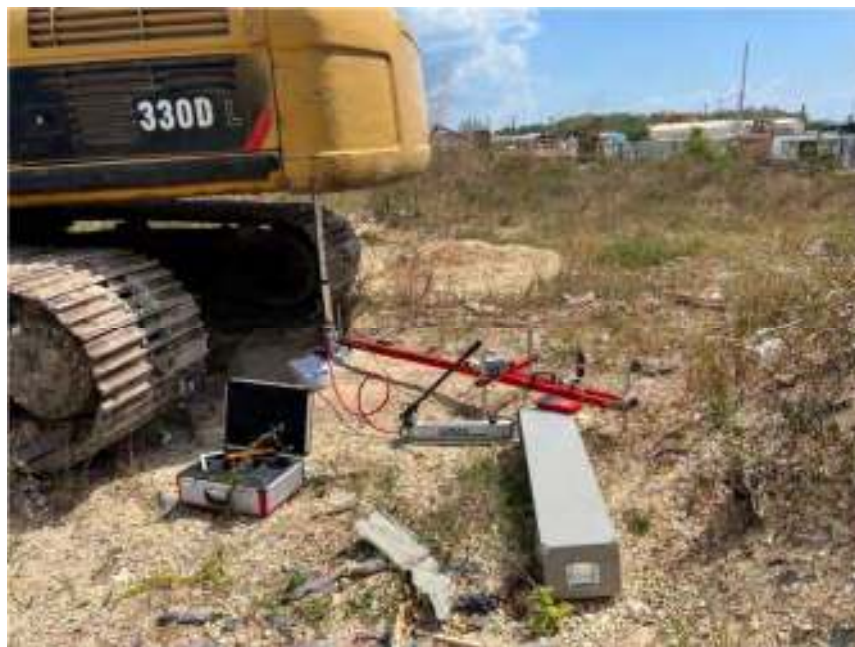
FIGURE A1 – PLT USING CAT330 AXEL AS COUNTERBALANCE
