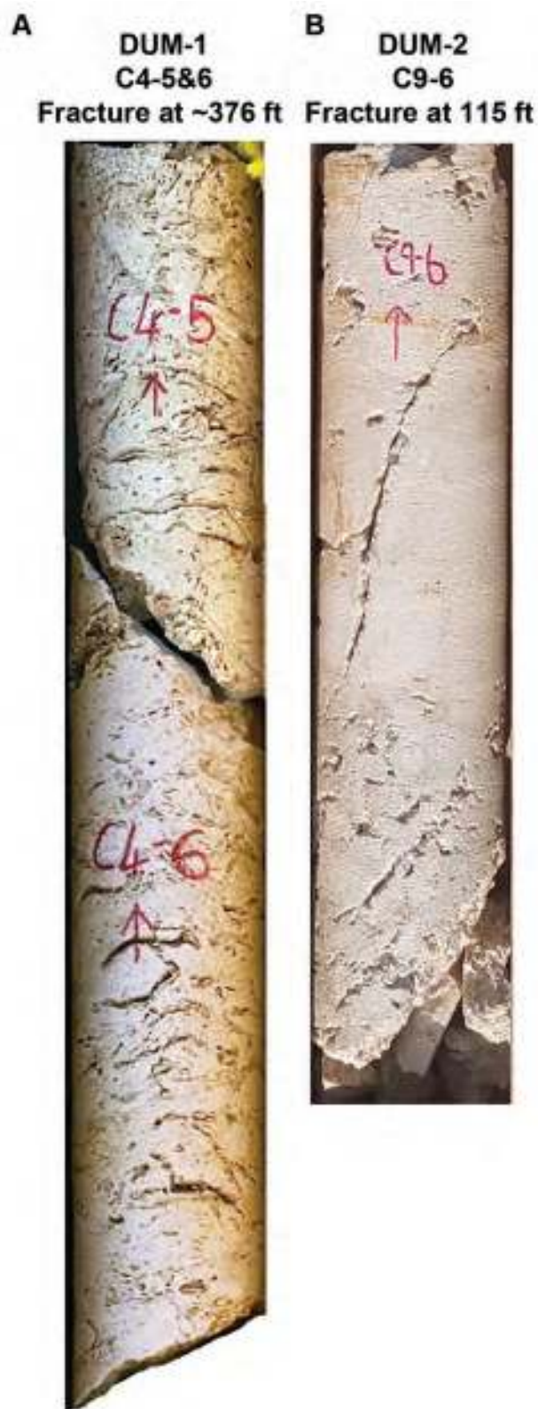
Figure 19. Examples of natural fractures in cores from wells DUM-1 and DUM-2 at depths of ~376 ft and ~115 ft, respectively. Core is 4 in (~10 cm) in diameter.
