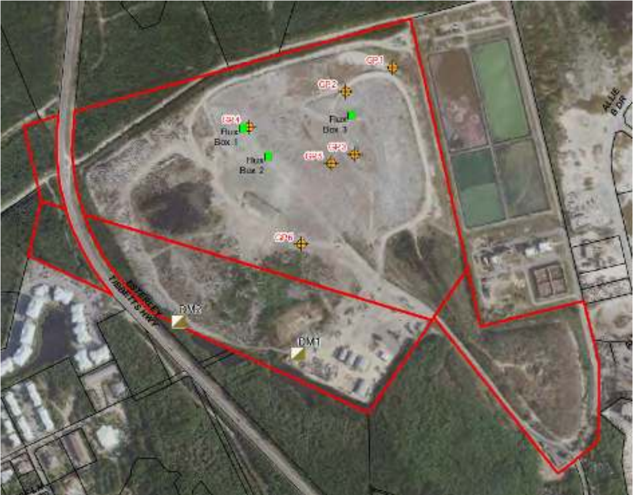
Figure 6 Location of the “gas probes” installed by Amec Foster Wheeler (2016b)
