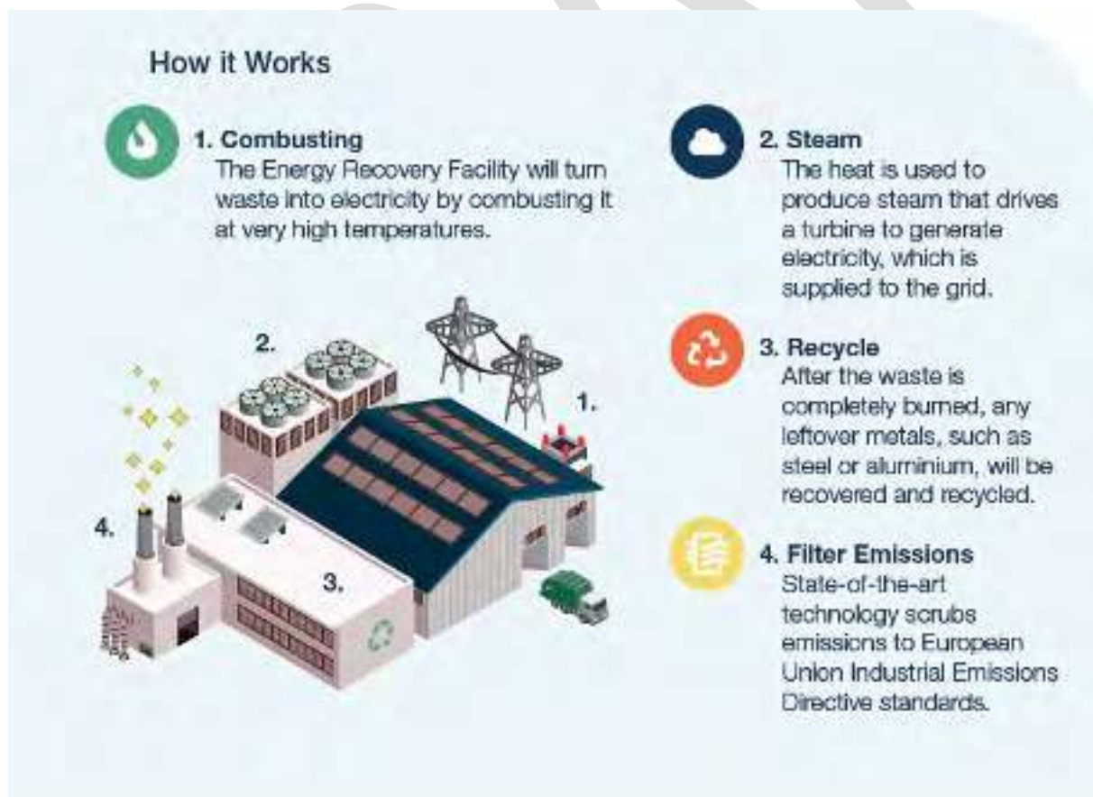
Figure 3.3 Energy Recovery Facility Process
