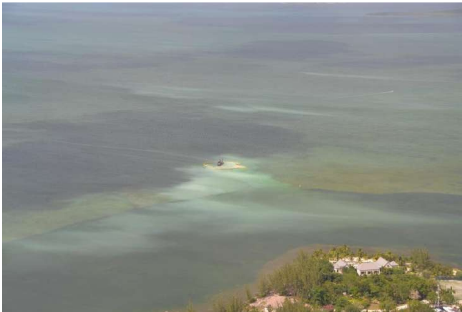
Figure 10: Monitoring photo from 28 April 2015 showing the sedimentation caused by the Harbour House Marina channel extension dredging project. This is the same dredging methodology currently being proposed. Note that silt screens were utilised but did not prevent the sedimentation from escaping.
