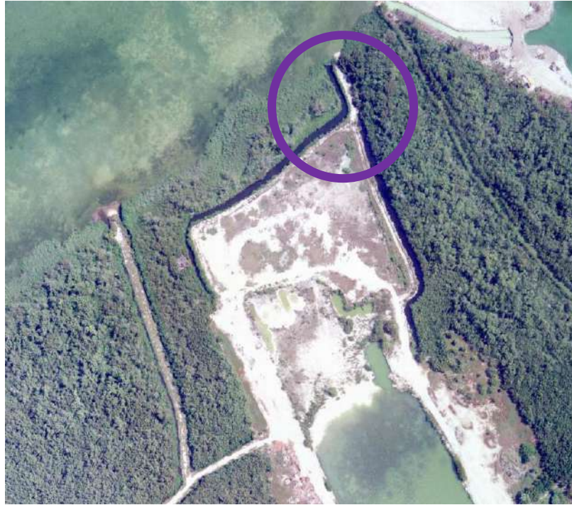
Figure 15: Cayman Land Info 1999 aerial extract showing the old dike road to the east of the property that could potentially be used to create a minimal flushing channel.
