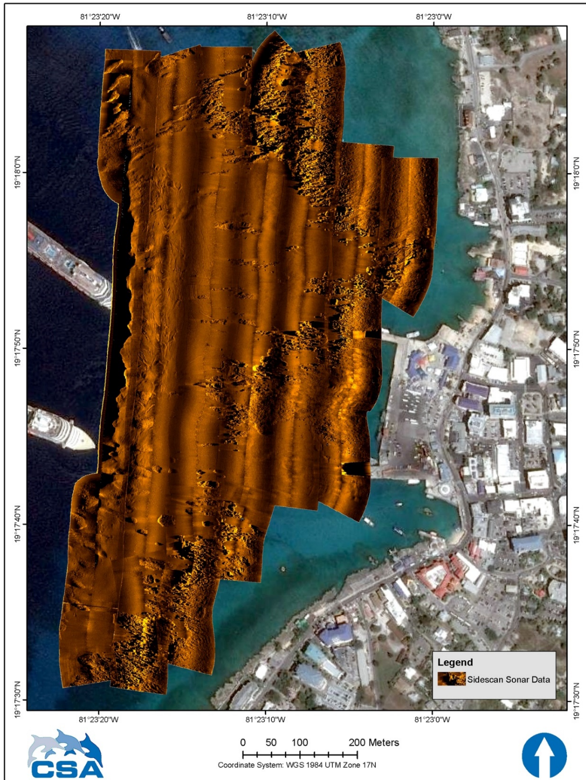
Figure 4. Mosaic of side-scan sonar data used to help document and map the distribution of consolidated and unconsolidated substrates within George Town Harbor.
