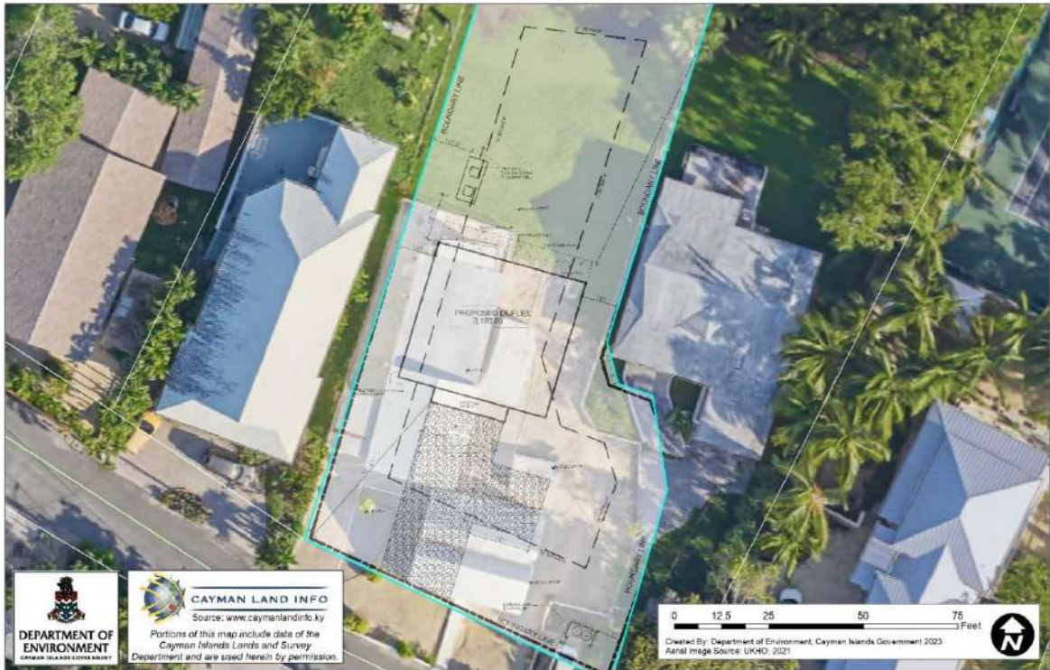
Figure 5. Proposed site plan overlaid on 2021 Aerial Imagery (Aerial Imagery Source: UKHO, 2021). Note that the footprint of the existing dwelling falls within the area of the proposed driveway / parking area.
