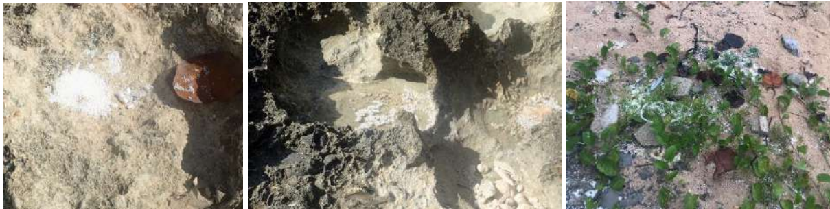
Figures 1-3: DoE site visit photos showing the bits of white polystyrene material littering local development sites. The beads from the first two images made their way into the adjacent Marine Reserve and neighbouring properties. Developers attempted to remedy the situation by cleaning neighbouring pools and yards daily but it was impossible to collect all of the beads, especially once they entered the marine environment.
