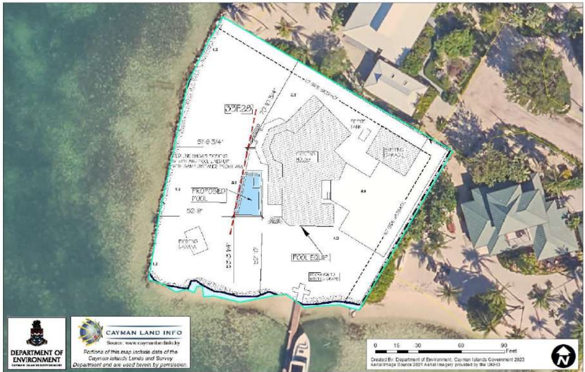
Figure 2: The proposed site plan overlaid on aerial imagery. The proposed setback for the pool falls short of the minimum required setback under the Development and Planning Regulations (2022 Revision) (Aerial Imagery Source: UKHO, 2021)
