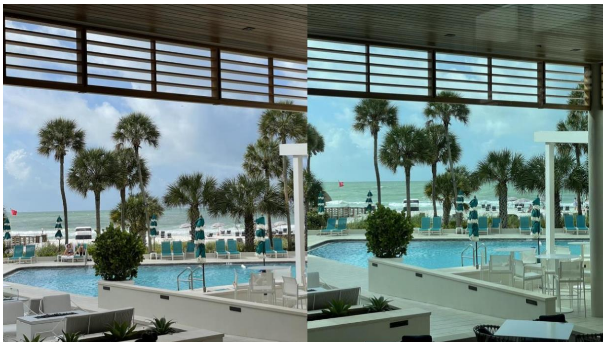
Figure 6. Looking out from a property with 100 VLT (i.e. no tint) on the left, versus 15% VLT after the retrofit on the right. Photos supplied by FWC.
