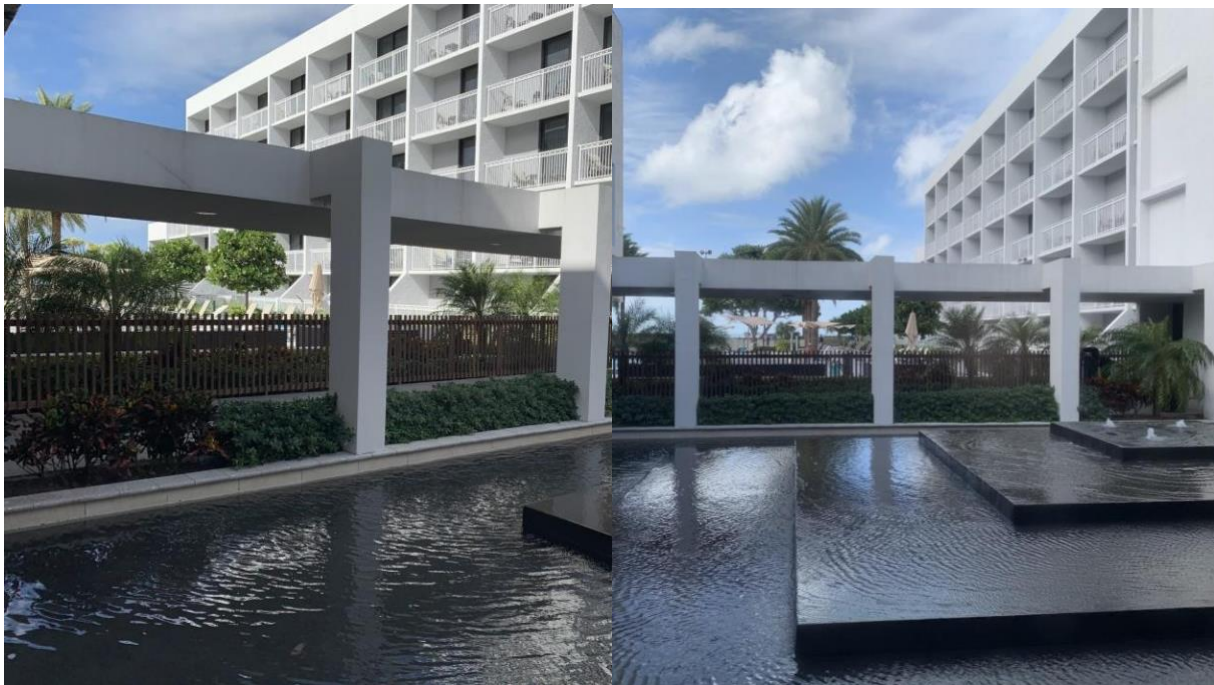
Figure 5. Looking out from a property with 100 VLT (i.e. no tint) on the left, versus 15% VLT after the retrofit on the right. Photos supplied by FWC.
