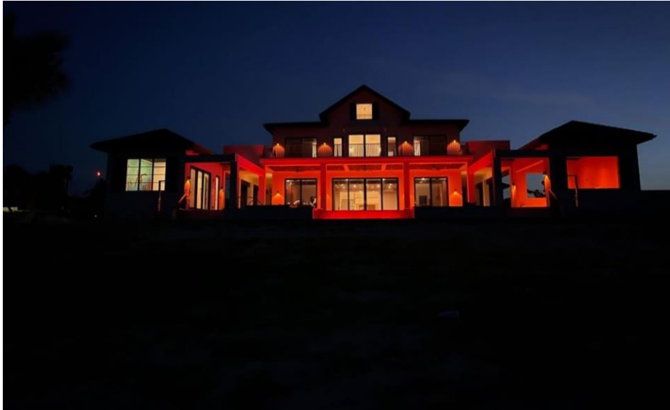
Figure 4. RipKai, which has 12% VLT tint, even though all interior lights are on, the beach in front remains dark.
