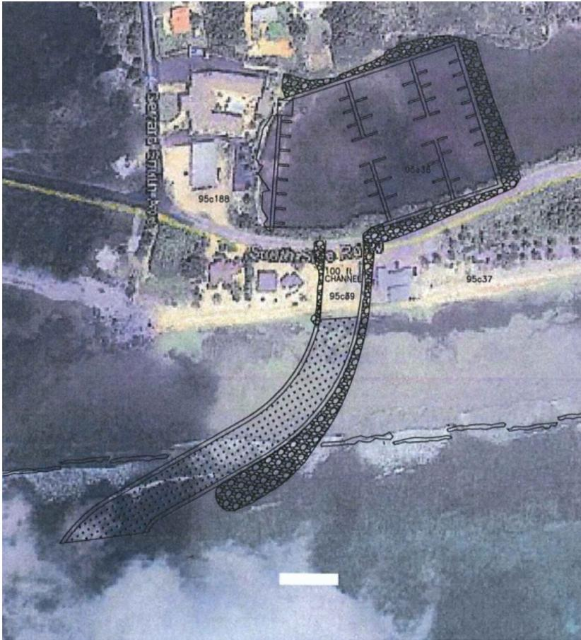
FIGURE 1: PROPOSED LOCATION OF CHANNEL AND ROCK GROYNES BREAKWATER.
